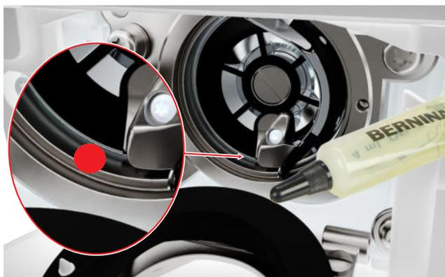
8. Hold the hook at the pin in the center with two fingers.
