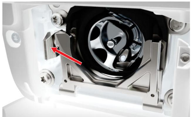
4. Fold down the fastening bracket with the black hook race cover.
