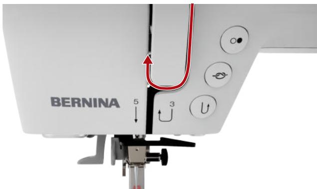
12. Guide the thread through the thread take-up lever and guide it downward. Make sure that the thread is guided under the left side panel.
