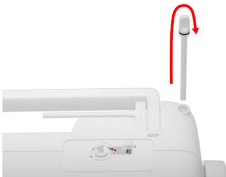
3. Place a foam pad and the spool on the vertical spool pin.
