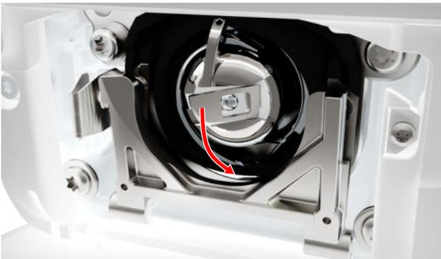
10. Insert the bobbin case. Hold the bobbin case by the tab so that the thread guide is pointing upwards.
