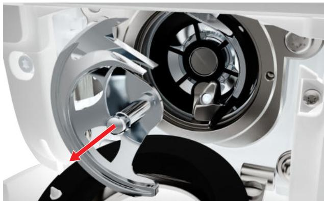
6. Clean the hook race area with a brush and a soft cloth. Never use any sharp instruments.
