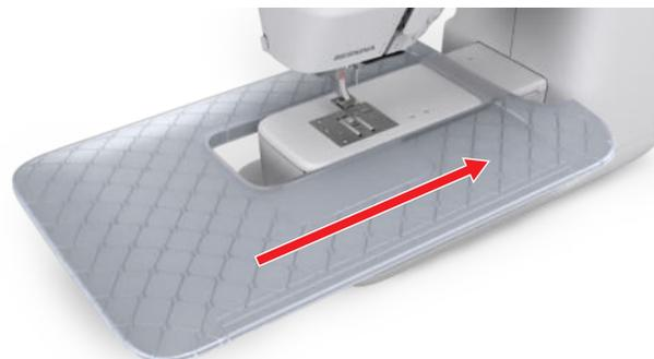
4. To remove the slide-on table, pull the slide-on table over the frearm to the left.
